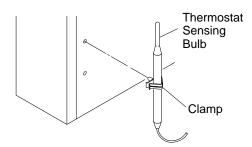
Figure 5 - Attaching Thermostat Sensing Bulb
